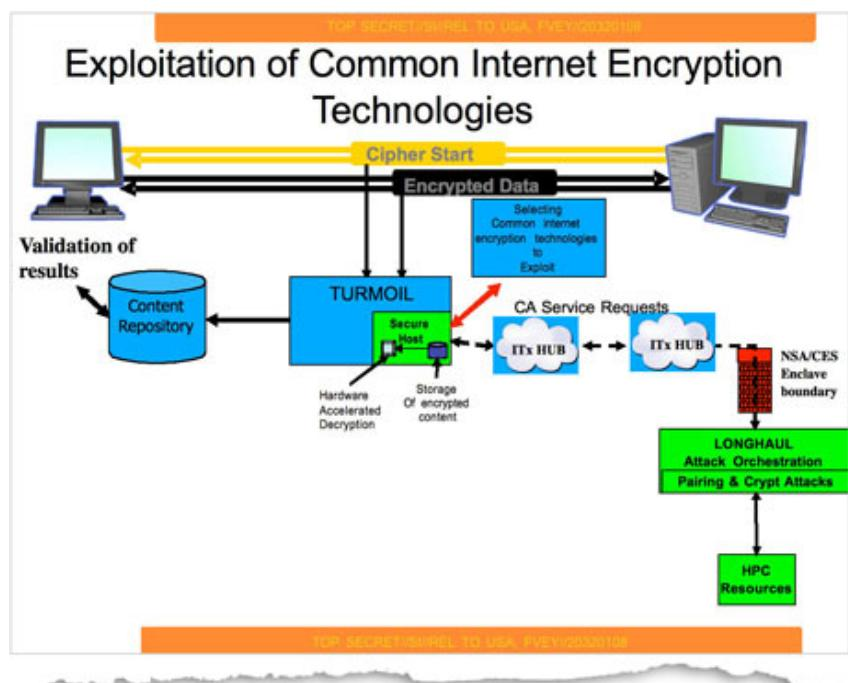
This network diagram, from a GCHQ pilot program, shows how the agency proposed a system to identify encrypted traffic from its internet cable-tapping programs and decrypt what it could in near-real time. Photograph: Guardian
