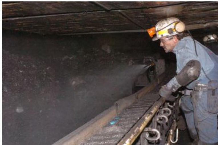
A longwall mining machine operator watches as the massive device cuts through a coal seam in a mine near Cameron, W.Va. Dale Sparks/AP
